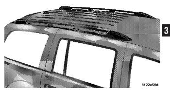
The load carried on the roof when equipped with a luggage rack must not exceed 68 kg (150 lbs.), and should be uniformly distributed over the cargo area.
